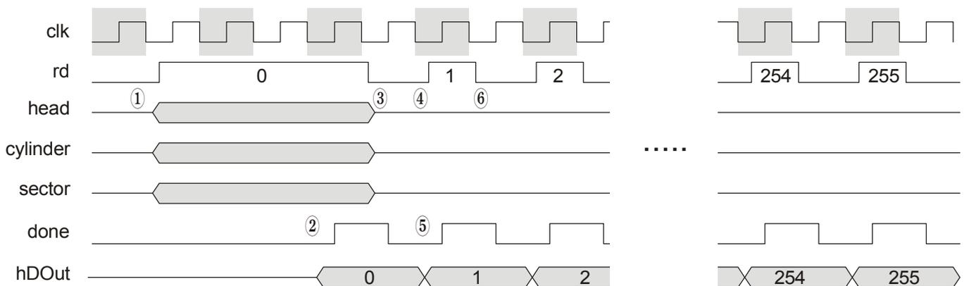
Figure 2: ATA controller read sector waveforms.
