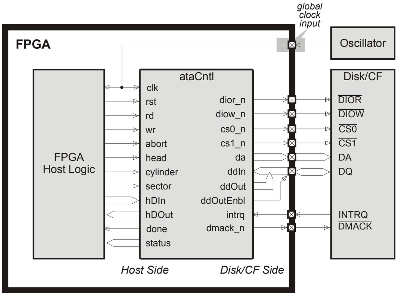
Figure 1: ATA controller connections.
