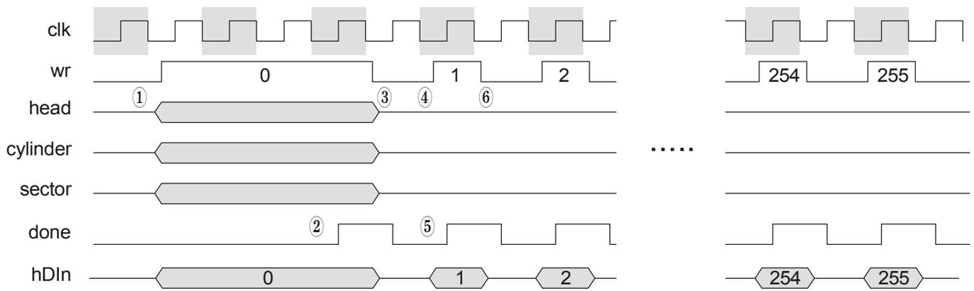
Figure 3: ATA controller write sector waveforms.
