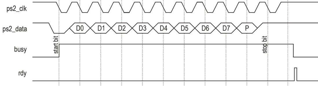
Figure 1: PS/2 keyboard waveforms.
