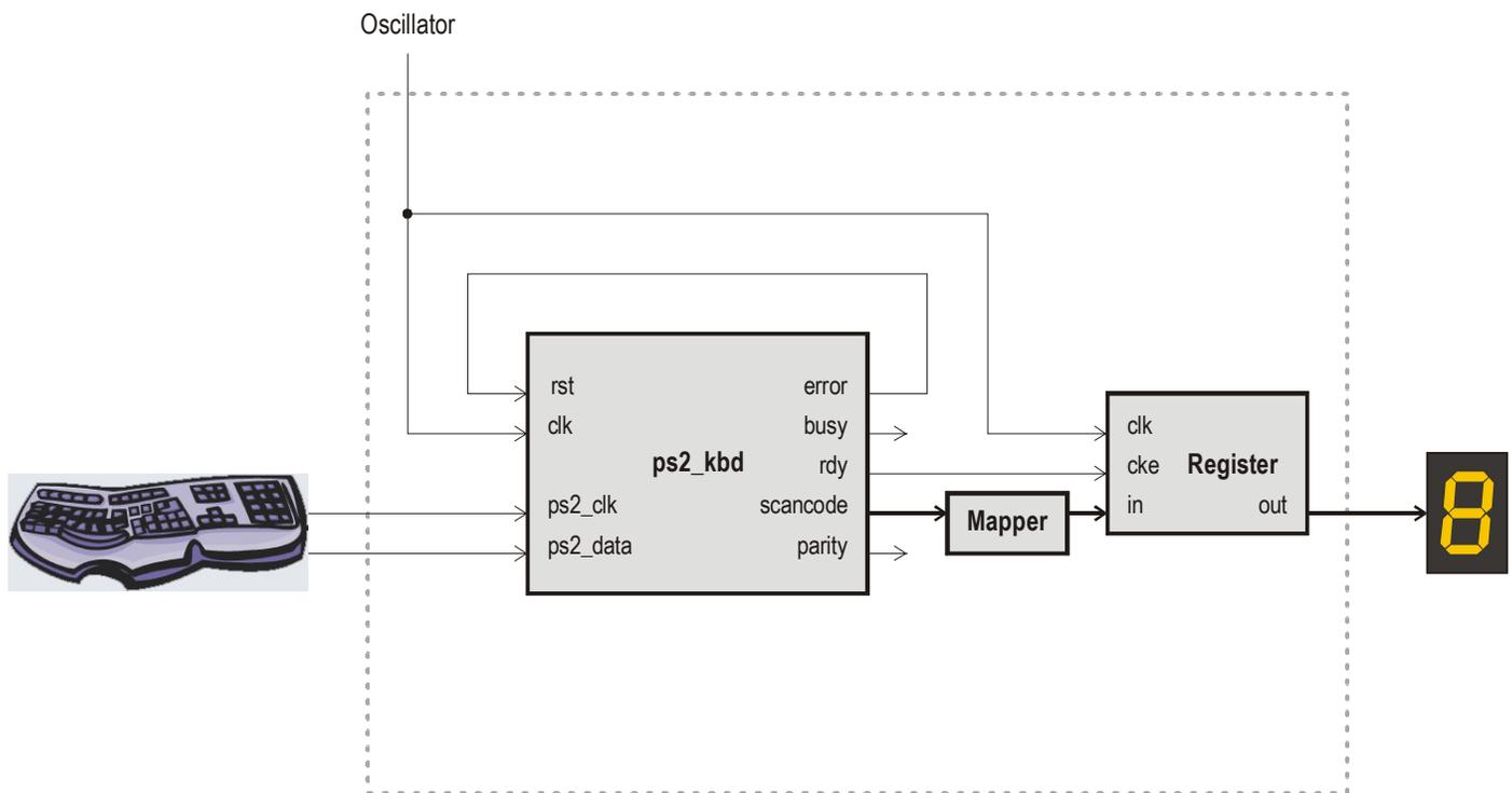
Figure 2: Using the PS/2 keyboard interface to display typed digits.
